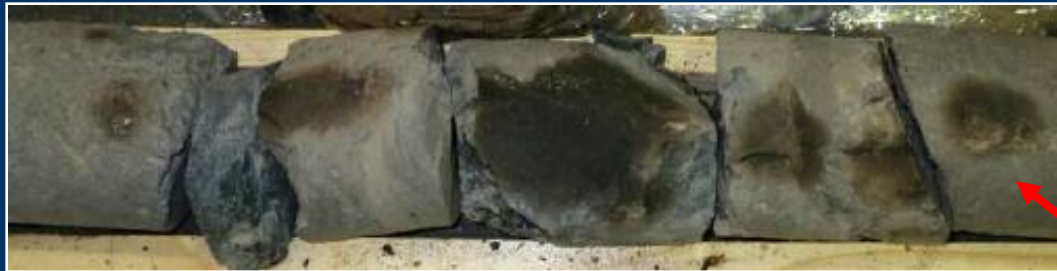
Core exhibits petroliferous odour upon extraction from core barrel
